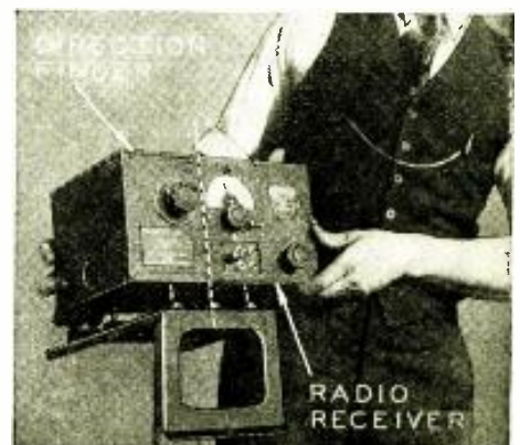
Below The Direct-Aire mounted alongside a Lear aircraft receiver makes a compact unit.
