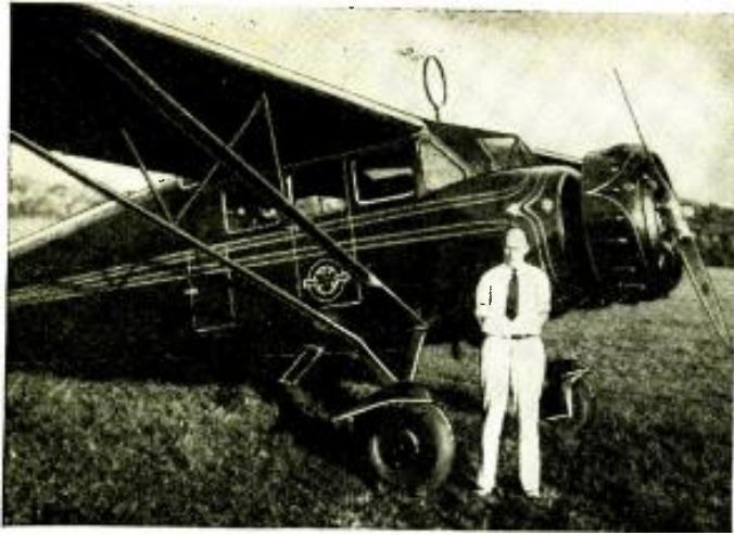
A directional-loop installation in a Stinson Reliant airplane. (Washington Inst. of Technology Photo)
