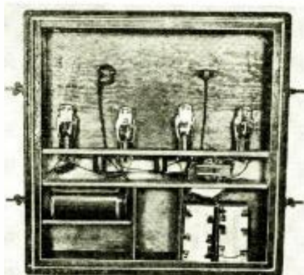
Fig. B Extra A.F. stage boosts signal.
